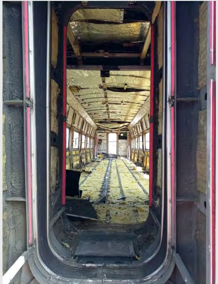
Figure 14-7: Train carriage following the removal of non-hazardous components, awaiting asbestos removal at a train dismantling facility in France
